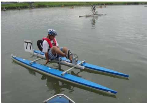
Photo1 human powered boat (made by FRP)
